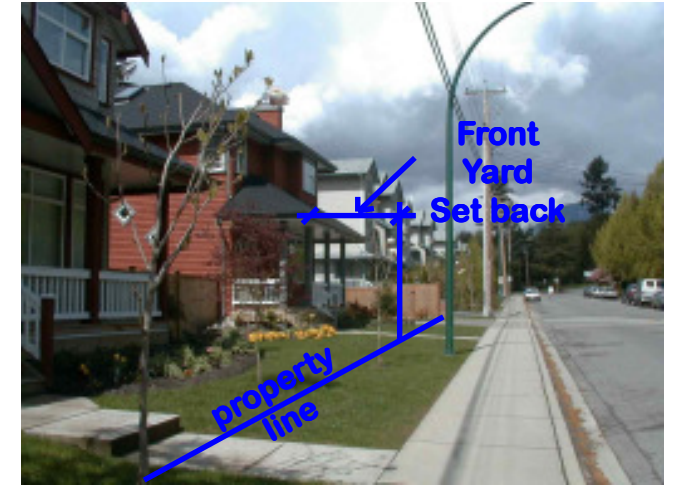
This photo of 989 Premier Street has the setbacks and property line marked on to illustrate how front yard setbacks are measured
