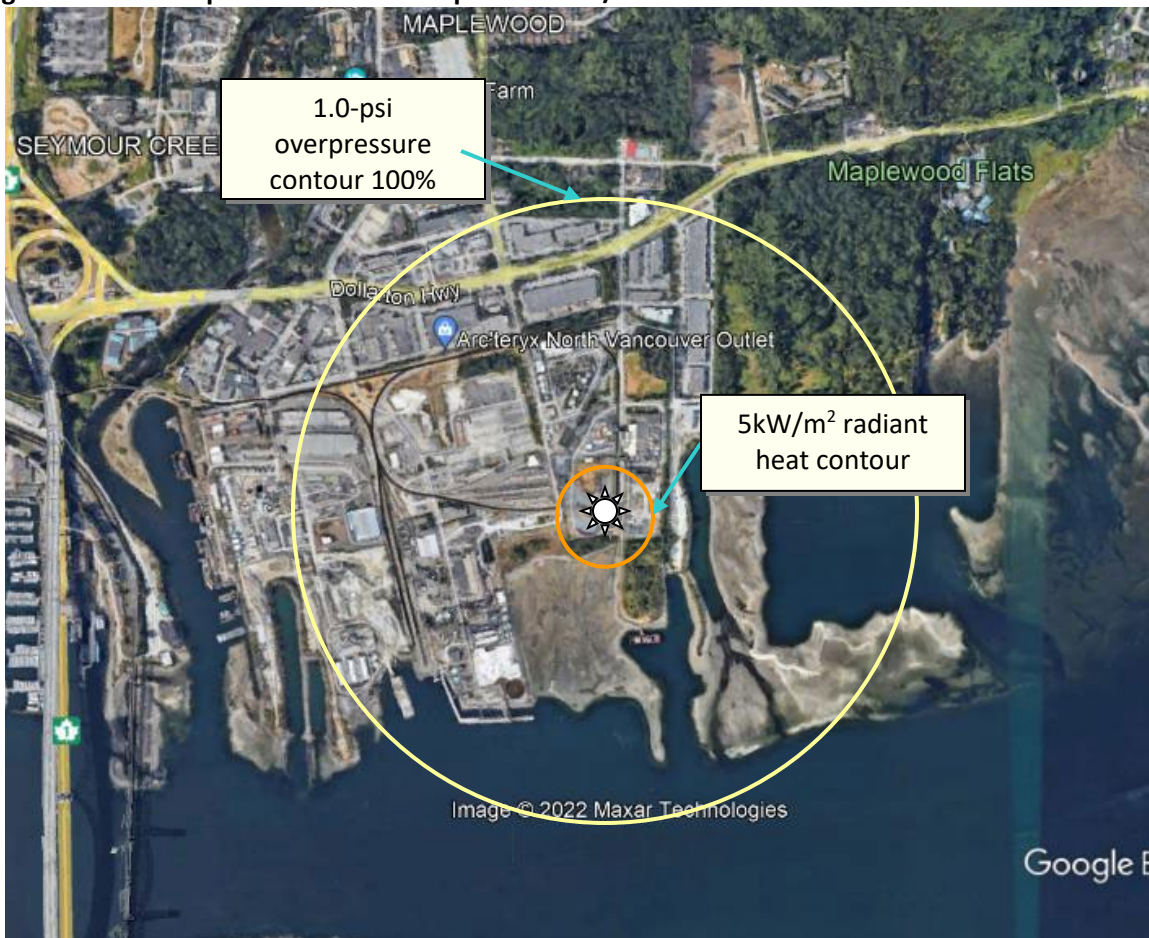
Figure 6: BLEVE Impact Distance to 1.0 psi and 5kW/m 2
