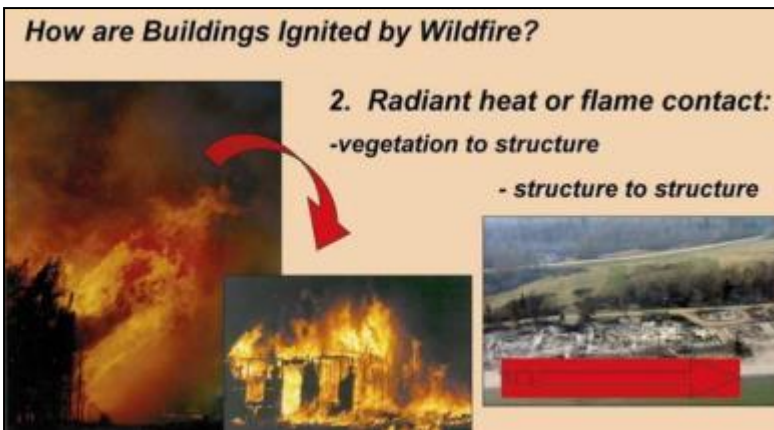
Figure 7. Radiant heat and flame contact allows fire to spread from vegetation to structure or from structure to structure.
