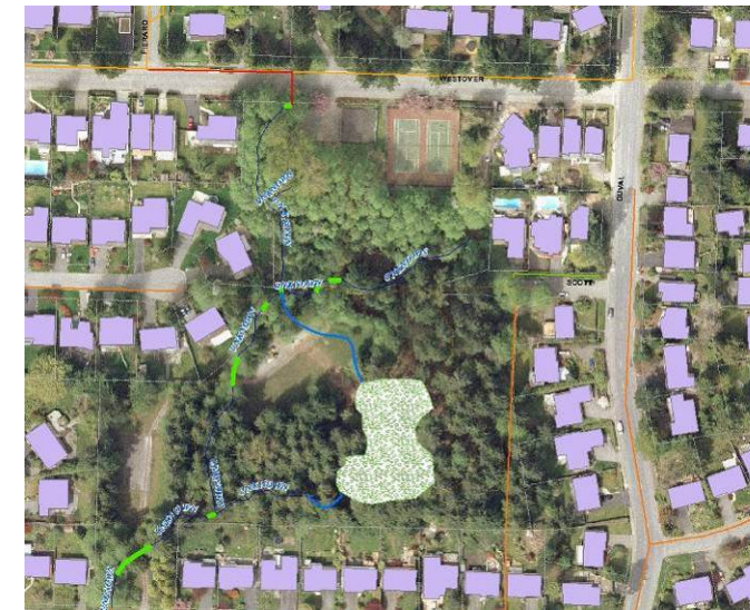
(g) Concept for attenuation facility in Draycott Park – some storm sewer work on Westover Road could move more discharge here.
