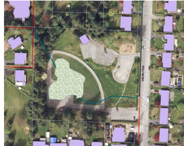
(b) Concept for LID facility at Viewlynn Park – proposed surface and subsurface facility with new stormmain along Viewlynn Road
