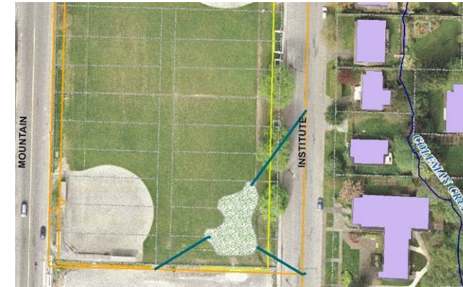
(e) Concept for LID facility at Lynn Valley Park – proposed surface and subsurface facility
