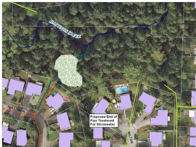
(c) Outfall from Princess Park (south) at Hunter Park – Proposed treatment wetland and possible off channel habitat
