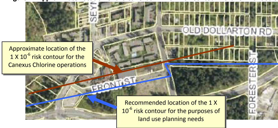
Figure 2: Approximate Location of the Canexus 1 \times 10^{-6} Risk Contour North of Front Street
