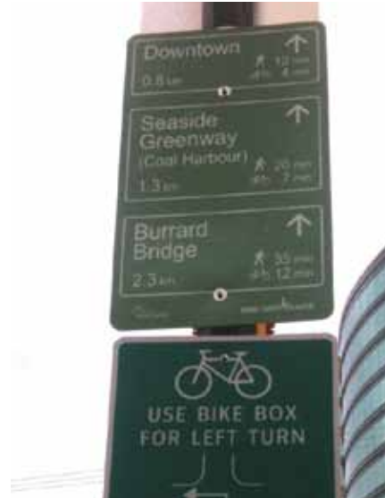
Left: Combining a lot of information on a sign aimed at different users can reduce legibility as a result of small text sizes and information overload.
