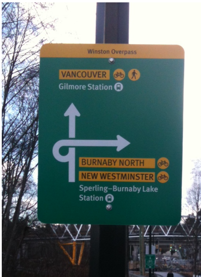
Prototype diagrammatic route sign developed for the complex Winston Overpass intersection of the Central Valley Greenway and local Lakes bikeway in Burnaby, BC
