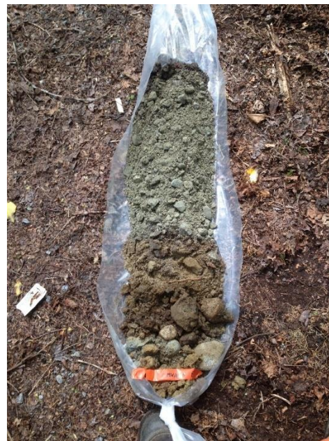
Photo 2. Coarse sand and gravel encountered in the borehole at MW16-06.
