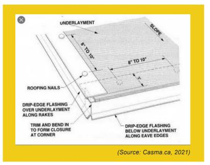
Eve-edge drip edging should be installed in the normal manner. Drip edge installed on rakes should be installed above the roofing underlayment to prevent water penetration beneath the underlayment.
